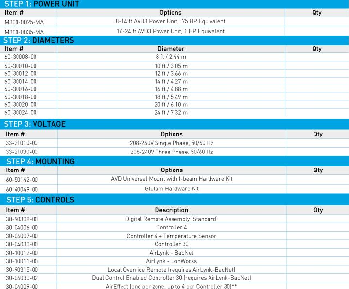
\*Motor unit only \*\*Only compatible with Controller 30, pricing is per zone. Not compatible with Dual Control option.
