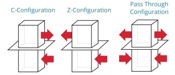
The Lift Configuration refers to the unloading and loading pattern of the lift. This lift allows for loading and unloading on the same side ("C"), from front to rear ("Z") or pass through.
