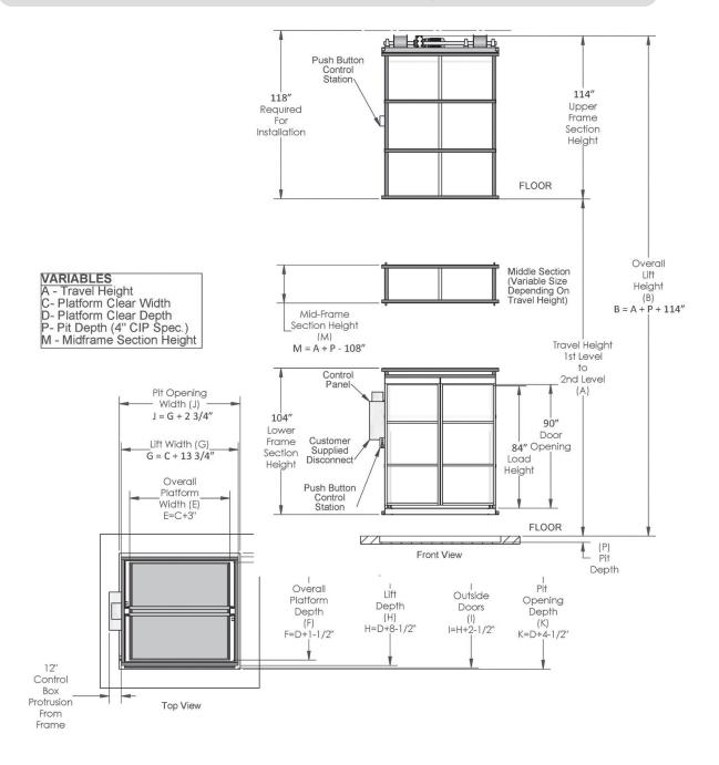
CIP Vertical Reciprocating Conveyors (VRCs) are manufactured to meet or exceed ANSI/ASME B20.1 Safety Standards for Conveyors and Related Equipment. This is the nationally recognized standard for vertical reciprocating conveyors. Proper installation is required to meet this standard. VRCs are not subject to ANSI/ASME A17.1 elevator codes unless specified, as they are designed for material lifting only.
