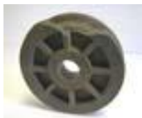
WORN CABLE ROLLER
